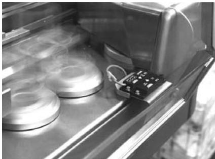
SMS safety magnetic sensors find their application field over a variety of cases: from extremely harsh industrial environments where really dirty and damp conditions are the rule up to applications where demanding hygienic standards are required and are met by the simplicity in cleaning the sensors, all of them being IP67.
