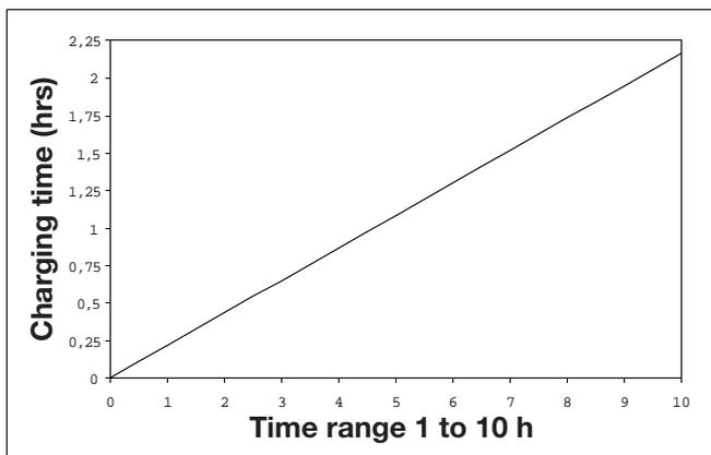
The tables indicate the charging time needed to keep the built-in battery fully charged for a certain adjusted time period.
