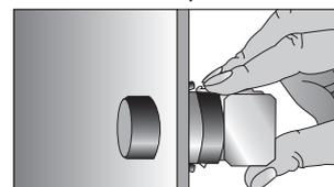
The contact block is snapped on.
