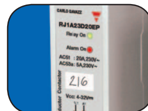
Identification window and LED indication of input status and optional over-temperature alarm status
