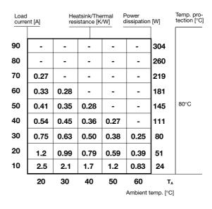
Compare the value found in the load current versus temperature chart with the standard heatsink values and select the heatsink with the next lower value.
