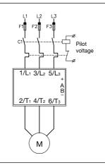
Overload protection by thermal relay
