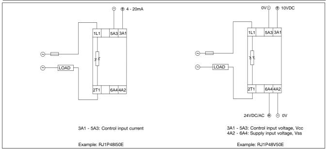
Note: For the RJ1P.V..., it is possible to have the ground terminals of the supply and control power supplies used commoned. In the case, this common ground is connected either to terminal A2 or terminal A3. This is only applicable when a 24 VDC supply voltage is used. There should be no external direct link from terminal A2 to Terminal A3.
