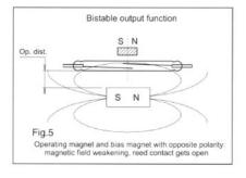
The **bistable** function can be carried out also with Change-over contacts, giving the Change-over / bistable function.
