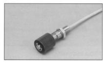
In this sensor a reed contact is operated by a float containing a permanent magnet. When the flux of the operating liquid pushes the float, the spring gets compressed and the magnet in the float causes the reed contact to switch. As the intensity of the flux decreases, the spring takes the float back to the rest position.
