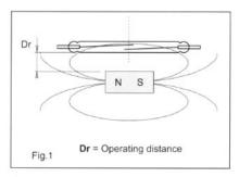
Magnetic sensors make use of reed contacts operated by means of an external magnetic field, generated by a permanent magnet (magnetic unit). A wide range of reed contacts is available with different features in terms of dimensions (standard or miniature), type (NO, NC, Change-over), electrical and mechanical properties, covering a huge variety of applications in the industrial filed.
