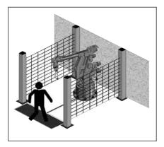
Safety module along with the SM-.. safety mat constitutes a safety system of safety category 3 in conformity with EN 954-1 and can be effectively used for a large number of monitoring exigencies also in harsh environments.
