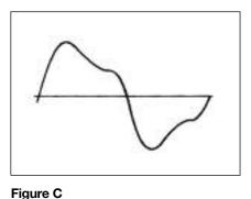
Sine wave, distorted Fundamental content 70...90% Harmonic content 10...30% Frequency spectrum: 3rd to 16th harmonic Additional error: <0.5% FS
