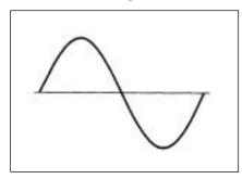
Figure A Sine wave, undistorted Fundamental content 100% Harmonic content 0% 1.1107 | A |  $A_{rms} =$
