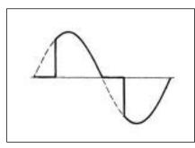
Figure B Sine wave, indented Fundamental content 10...100% Harmonic content 0...90% Frequency spectrum: 3rd to 16th harmonic Additional error: <1% FS
