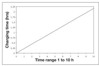
The tables indicate the charging time needed to keep the built-in battery fully charged for a certain adjusted time period.
