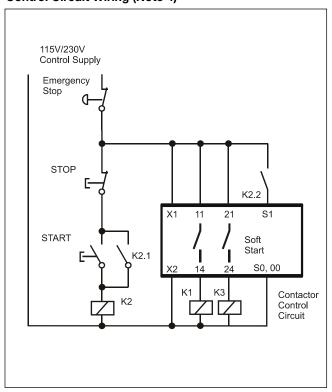
Note 4: Contactor K3 is required for the 'operation in Bypass Power Circuit' and is controlled by the programmable relay set as 'Top of Ramp' relay.
