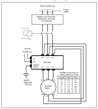
Note 2: The In-Delta configuration requires that the firing mode be set to '1'. An in-line contactor controlled by the RSXK MUST be used in the In-Delta firing mode.
