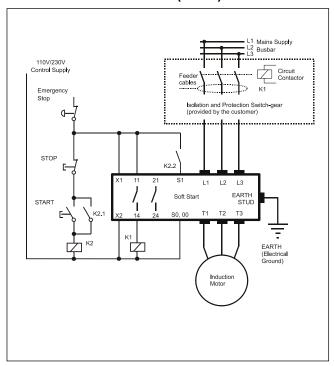
Note 1: The in-line configuration shown above requires that the firing mode be set to '0'.
