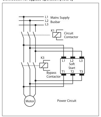
Note 3: The bypass configuration is automatically detected as "Auto Bypass" is set as default.
