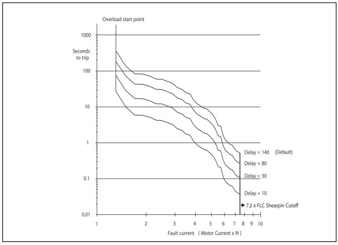
Current Limit', 'Overload level' and 'Overload delay' settings may be adjusted to limit overload currents in accordance with the trip curves shown here. For motors with FLC's lower than the rated current of the RSQK, the 'Overload Level' may be adjusted using the following formula: Overload level = Motor FLC x 1.1 (A)
