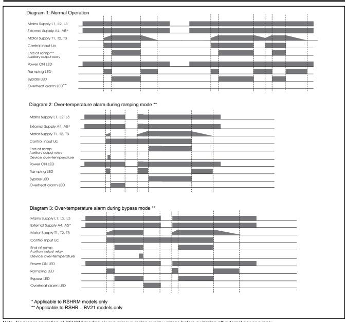
Note: for proper operation of RSHRM models always remove mains supply voltage before switching off external power supply.
