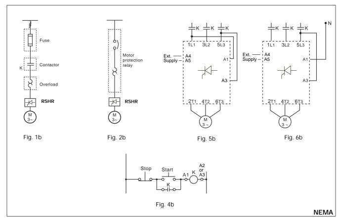
The motor controller provides by-passing of the semiconductors during running operation. Therefore the semiconductors can only be damaged by short-circuit currents during ramp-up and ramp-down. Please note that the motor controller does not isolate the motor from the mains
