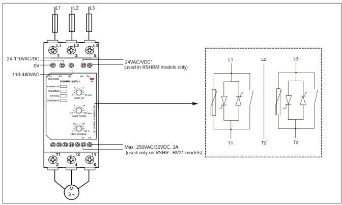
$<sup>^{\</sup>star}$  For the 24VDC external supply, CG power supply model SPD24051 can be used
