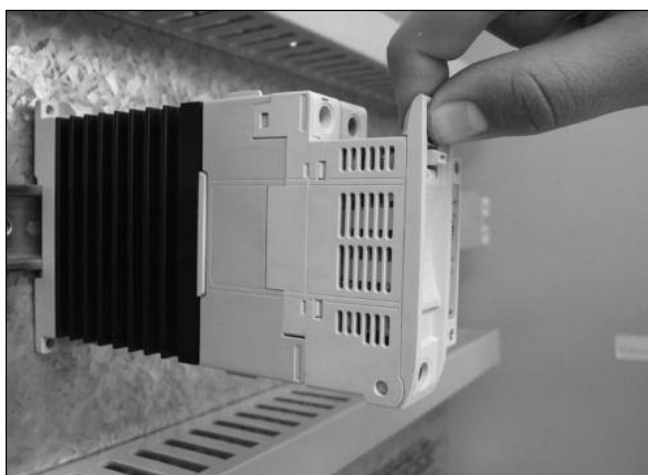
1. Preparation for opening fuse holder.
