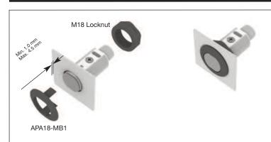
PA18 mounting with a combination of 1 x APA18-MB1 and 1 x M18 locknut.
