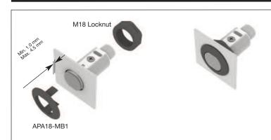
PA18 mounting with a combination of 1 x APA18-MB1 and 1 x M18 locknut. Maximum torque  $0.9 \ NM$
