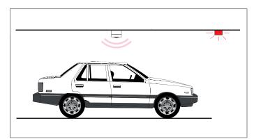
better solution in terms of visibility to use a slave LED indicator mounted externally along the carpark driveway. The sensor is equipped with a Dupline® 3-wire bus interface for power supply and communication.
